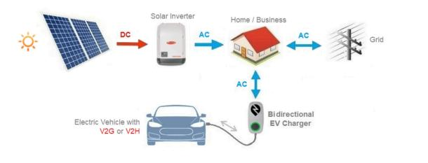
Figure 13. Bidirectional EV Charging
