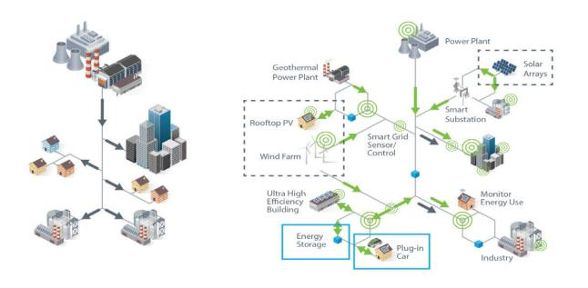
Figure 7. The Existing One-Way Grid Architecture and the Digital, Decentralized Grid Architecture
